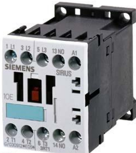
CONTACTOR, AC-3 3 KW/400 V, 1 NC, DC 24 V, 3-POLE, SIZE S00, SCREW CONNECTION
